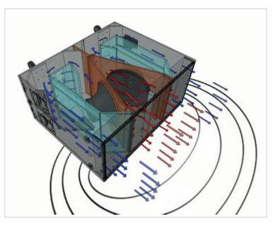
an over-damped reflex load. Moreover, the maximization of the mutual coupling between the drivers increase the fastness of the transient response while maximizing the overall energy efficiency as well.
